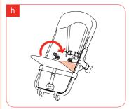
Attach the 2 hook and loop fasteners at the foot end to the underneath the frame.
